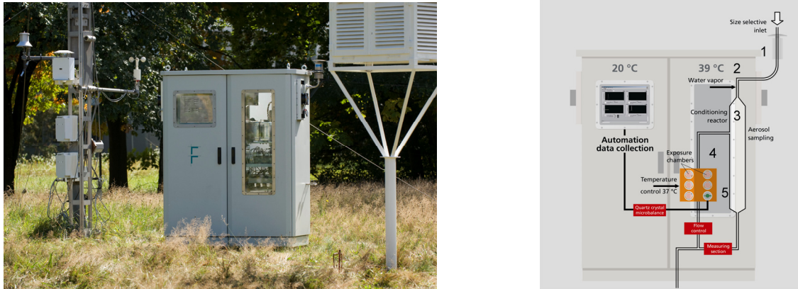
Figure 4.1 Right: Scheme of the Cell Exposure System with the (1) size selective inlet, (2) the water vapour dosage for humidification (3), the conditioning reactor for a constant aerosol with 37°C and 85% r.h., (4) the VITROCELL® exposure chambers containing the Transwell® membrane inserts and the sensor of the (5) quartz crystal microbalance. Left: photograph of the fully automated and temperature controlled prototype during an outside measurement of environmental aerosols.
