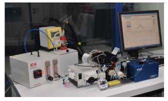
Figure .1. The developed DIPNA breadboard system
