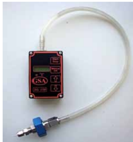
Figure 8. Pre-prototype CNT specific sampler by Fraunhofer IPA.
