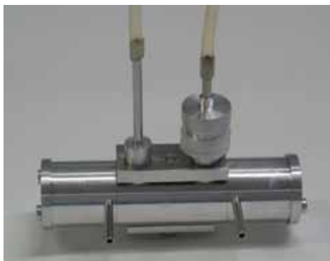
Figure 7. Extra-thoracic region (ET1) modular pre-separator developed by University of Lund
