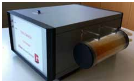
Figure 1. Electrical and optical (pre)-prototype to measure particle size distribution, total number concentration, surface and volume distribution, total surface and total mass fractions. Developed by GRIMM
