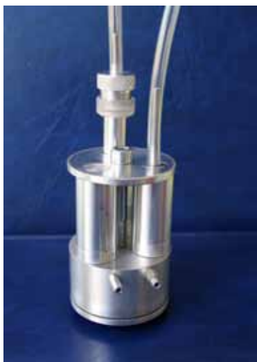
Figure 6. Gas-exchange region (GE modular) pre-separator developed by University of Lund
