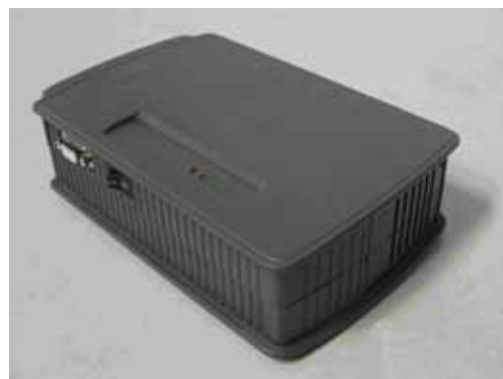
Figure 2. Pre-prototype instrument to measure particle size developed by DEKATI and TUT
