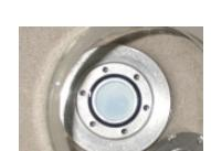
Target holder with activated TiO<sub>2</sub> NPs
