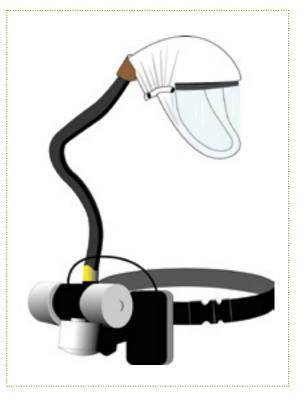
Personal protection measures: schematic drawing of a power air purifying respirator (PAPR)
