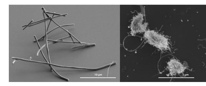
Open cluster (left) and agglomerate with single fibres (right) of nanoscale material. Pictures were taken with a scanning electron microscope (SEM).
