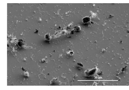
Scanning electron microscope (SEM) picture of carbon nanotube agglomerates and single fibres.
